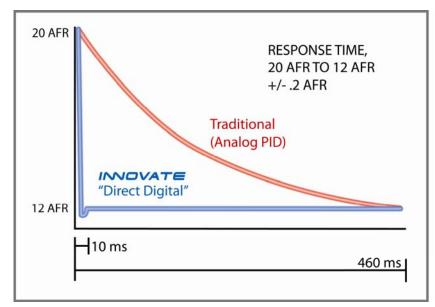
In a conventional PID feedback wideband controller the temperature is regulated via the AC impedance of the reference cell (usually measured with a small AC current of 1-4 kHz). This measurement frequency has to be filtered back out of the reference cell signal with low pass filters and that cause further latency in the measurement loop.
