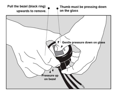
🔥 Pulling bezel upwards while NOT not holding the glass down can 🕂 potentially damage the gauge.
