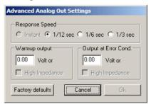
When setting the MTX-OL PLUS to the slower response speed settings, the measured mixture data will be averaged over the response time setting before being sent via the analog output.
