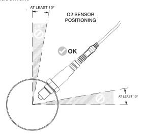
Tightening Torque - 33-44ft/lbs (45-60Nm)
