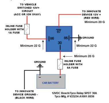
NOTE: Use of a relay is not required for installation but can be helpful in providing clean power, particularly if your vehicle has limited options for key switched power.
