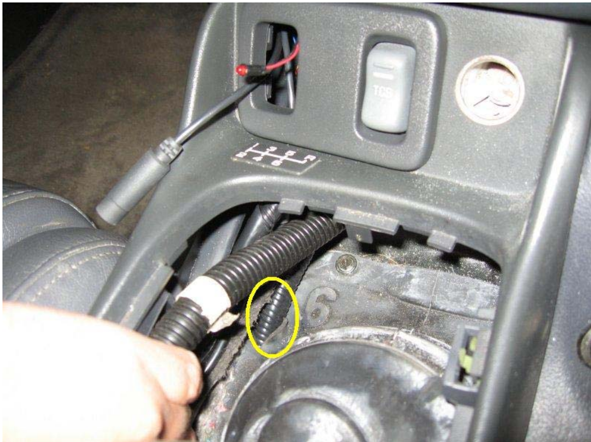
Picture 4: LC-1 Cable Routing (Cables in Wire Loom)
