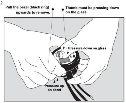
\* When disassembling, be careful not to lose the clear plastic light pipe from the warning light opening as it can fall out.
