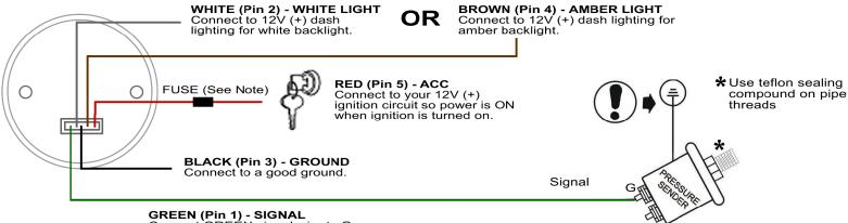
**GREEN (Pin 1) - SIGNAL**Connect GREEN signal wire to G terminal on the pressure sender.
