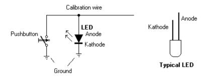
Note: The LED will fit a 5/32" (0.155" - 0.158") hole size and a panel thickness of 28–16gauge (0.031" - 0.062").
