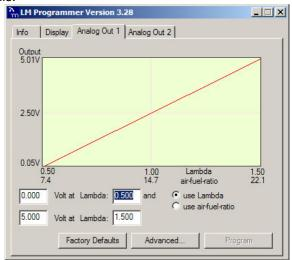
This shows the analog output voltages versus Lambda for one of the two analog outputs. The graph display is automatically scaled to the selected voltages. For each output you can specify a minimum and maximum lambda or A/F ratio value and the associated voltages.
