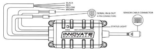
1. Status Light – The LC-2 status light indicates the controller's operational status. When the controller is powered, the status light will light up green for 2 seconds indicating controller initialization.
