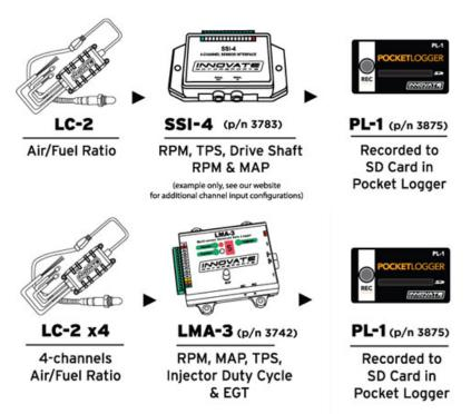
Innovate Motorsports' MTS devices have two types of serial interface connectors, the legacy 2.5mm stereo and the 4 pin Molex. The following patch cables are available to interface your devices together:
