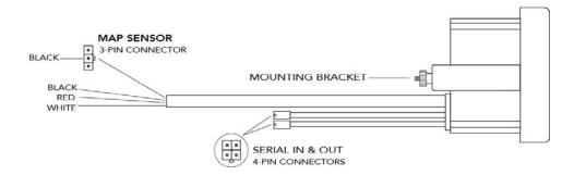
1 Connect the RED wire to an isolated switched 12V source in your vehicle. A switched 12V source goes ON as soon as "key on" power is active. The circuit to which you will pull power from should be able to support a 2 amp draw. Make sure this connection is protected with a 5A fuse.
