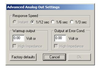
When setting the MTX-AL to the slower response speed settings the measured mixture data will be averaged over the response time setting before being sent via the analog output.
