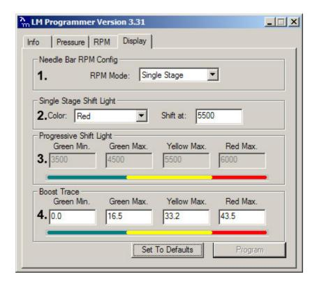
1. **Needle Bar RPM Config:** You are able to select between Single Stage or Progressive shift light.
