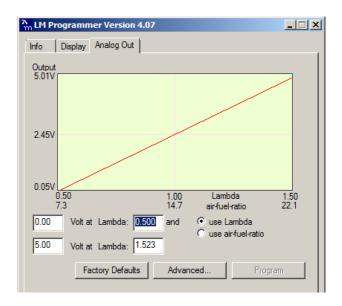
This shows the analog output voltages versus Lambda for the analog output. The graph display is automatically scaled to the selected voltages. You can specify a minimum and maximum lambda or A/F ratio value and the associated voltages. Below the minimum and above the maximum values the output voltages stay constant at the associated programmed voltage.
