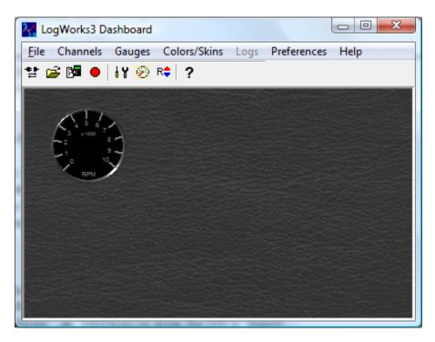
3. Select "Connect", either the leftmost icon on the toolbar (it is supposed to be a male and female socket with arrows in both directions below) or select "Connect" from the "File" menu. A box like this should appear:
