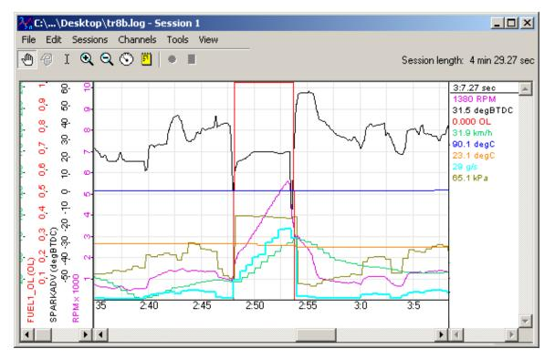
This extra resolution comes at the expense of our Low Priority inputs. These channels all share the ECU 'bandwidth' once used by VSS alone. But, this lets us have high resolution critical data combined with lower priority, lower resolution data in the same log.
