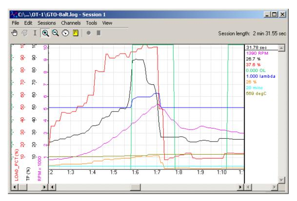
Like the Saturn, it is connected using 500K bit CAN, but we can begin to see some 'steppiness' in the RPM channel with only 8 channels being collected. In addition, some values, like the Calculated Load are courser still. Presumably because the ECU itself is only calculating them a few times per second.
