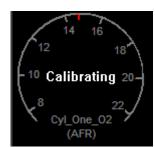
The Heater Calibration and Free Air Calibration are unique to each sensor. If you use a different sensor on a LC-1ST you will need to run through the whole Calibration procedure again (section 3.2)!
