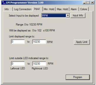
As you can see here, the display will indicate in 100 RPM. This might be too coarse for many applications. The limit is there because the XD-16 can only display 3 digits. By applying a limit (for example to 0...9990 RPM the
